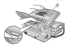
4 Hold the center part of the front cover (1), and pull open the inner cover (2).
